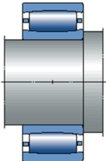
Reoccurring temperature faults within the generator caused by lubricant failure and lack of protection of the bearings can result in downtime and the loss of power generation. Bearings can reach temperatures of above 150°C. Most standard industry generator greases are not rated to operate at such high temperatures. FUCHS URETHYN XHD 2 is designed to handle temperature spikes up to 180°C and provides for user safety margin when it comes to high temperature.
