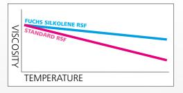
As there is no industry standard for fork oils each manufacturer has a different viscosity for their own particular "wt" oil. We have decided to move away from the use of weight
