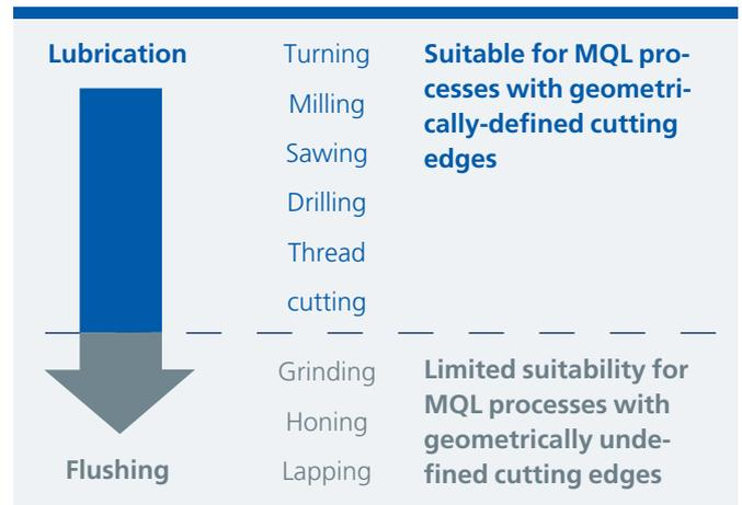
**PLANTO MIKRO and ECOCUT MIKRO PLUS products are suitable for use with single-channel (AEROSOL BUSTER) and/or two-channel spray systems.**
