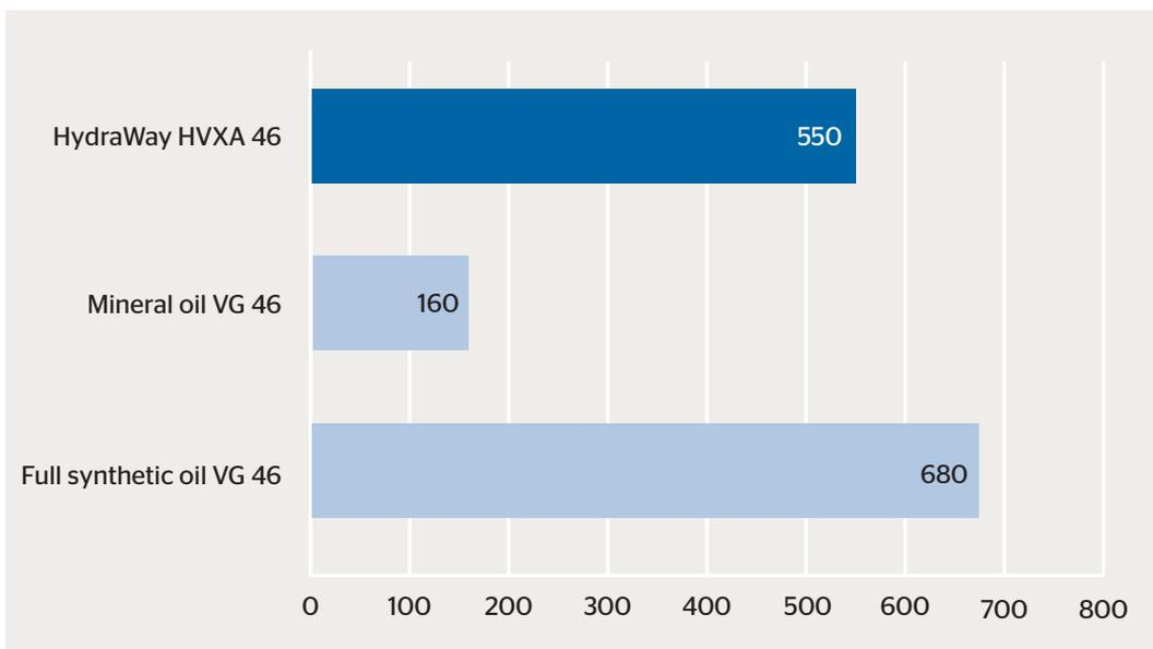
HydraWay HVXA 46 has oxidation stability 3 times higher than ordinary mineral hydraulic fluids and slightly lower than high priced full synthetic hydraulic fluids.
