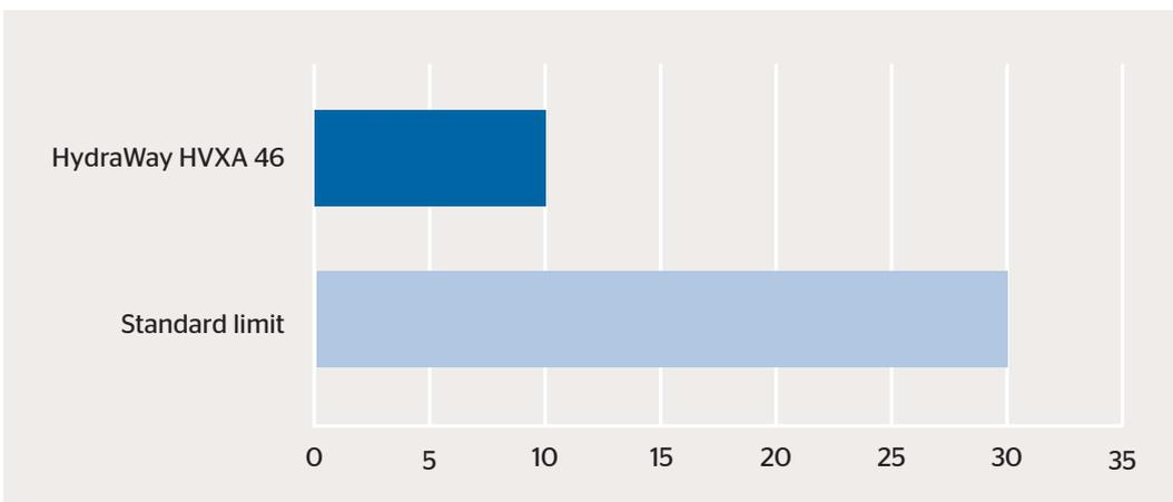
The HydraWay HVXA series has very efficient demulsibility which is 3 times better than standard DIN 51524 part 3, ISO 11158 HV requirements, which makes it ideal for application in mobile equipments that are used outside.
