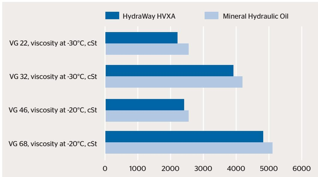
HydraWay HVXA series hydraulic fluids can be used in much colder conditions than the same viscosity grade from competitors.
