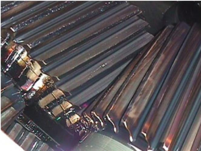
Gear before the change over to GEARMASTER ECO 320
