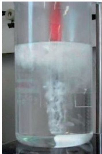
Figure 4: PAG-collapse of the vapour phase (concentration > 20 %)
