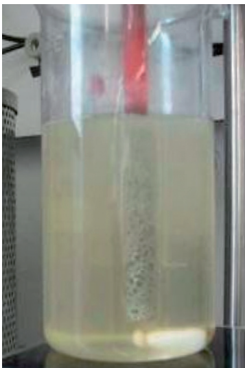
Figure 5: PVP collapse of the vapour phase
