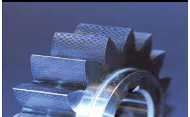
Figure 1: test gear after DIN wear test, no wear, manufacturing marks still visible
