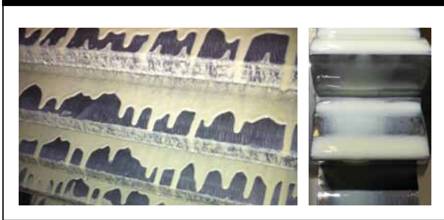
Figure 2: left – lubrication film after a 6h shutdown of a cement mill with spray application and right – retention of lubrication film after a 21-day lab test
