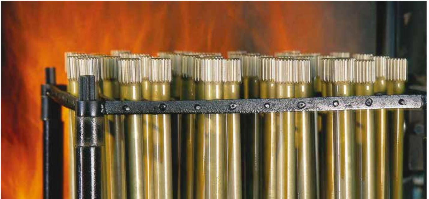
When selecting the most suitable high-performance quenching oil for a particular application, an initial rough differentiation can be made between high-viscosity and low-viscosity quenching oils.
