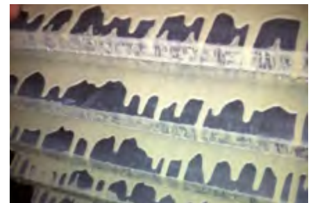
Lubrication film after 6 hours downtime
