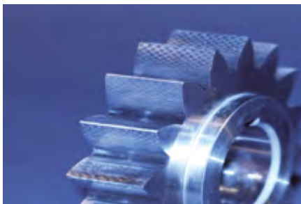
Test gear after DIN wear test / no wear / manufacturing marks still visible
