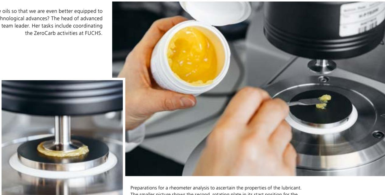
Preparations for a rheometer analysis to ascertain the properties of the lubricant. The smaller picture shows the second, rotating plate in its start position for the measurement. Then the black cover is lowered, meaning that you can no longer see the measurement plates. The cover ensures that the temperature can be regulated to predefined values.
