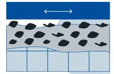
Partial separation of solid lubricant from the SFL
