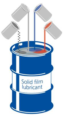
After drying and curing solid film lubricants form a dry lubricant film of a few microns reliably adhering to the base material. This film acts as a friction- and wear-reducing, separating and lubricating layer between the friction partners.
