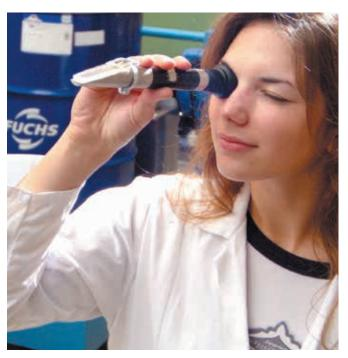
When using a hand-held refractometer, it is important to set the zero point adjustment with pure water prior to any concentration measurements. A heavily contaminated or less than stable emulsion or one which has excessive tramp oil can lead to the dividing line being diffused which, in turn, caused inaccurate or unsafe concentration measurements.
