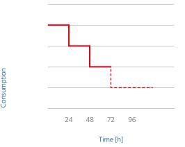
Note: The attainable minimum quantity is directly subject to the operating conditions. Lubrication rates below the minimum may create an increased risk of wear and damage on the tooth flanks.
