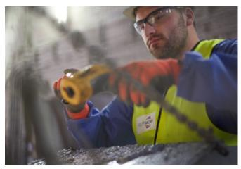
Dynamic check of the contact pattern with a stroboscope
