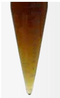
Commercial PAO Wind turbine gear oil VG 320 after storage
