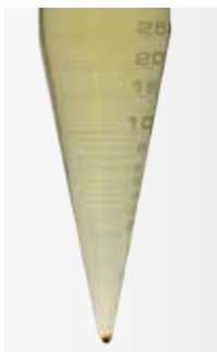
Afterwards the oils are tested on deposit formation by diluting with solvent in a centrifuge tube.
